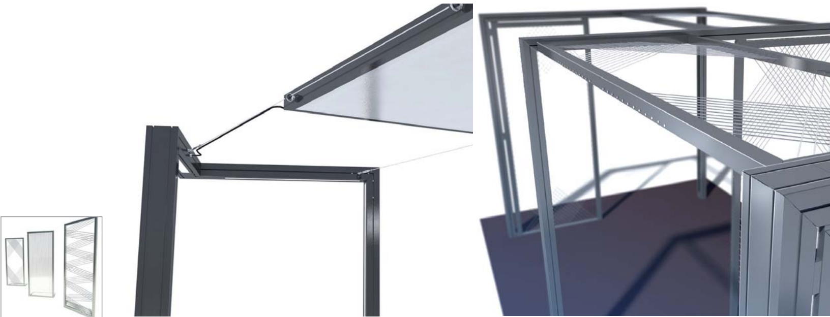
Cadres additionels Éléments lumineux supports de textures, fixés aux modules techniques, permettant de varier les atmosphères Additional frames Lighting texture supports elements, fixed to the technical modules to enhance the lighting atmosphere
